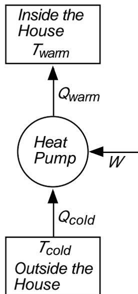
represented by the circle in the middle of the diagram. The cold environment outside the house is represented by the box at the bottom, and the *absolute* temperature of that environment is denoted by  $T_{cold}$ . The warm environment inside the house is
